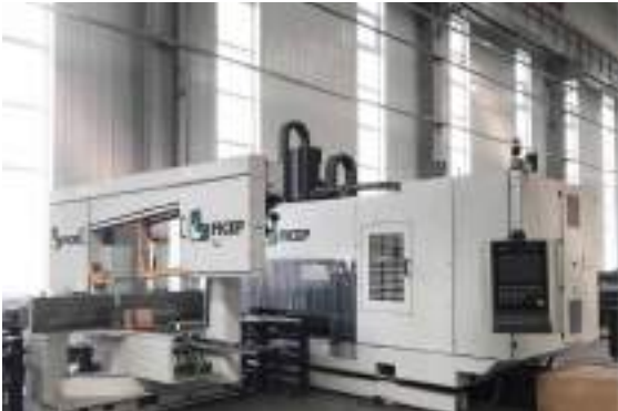
意大利菲赛普FICEP钻锯联合生产线 Italian FICEP joint production line of drilling and sawing
